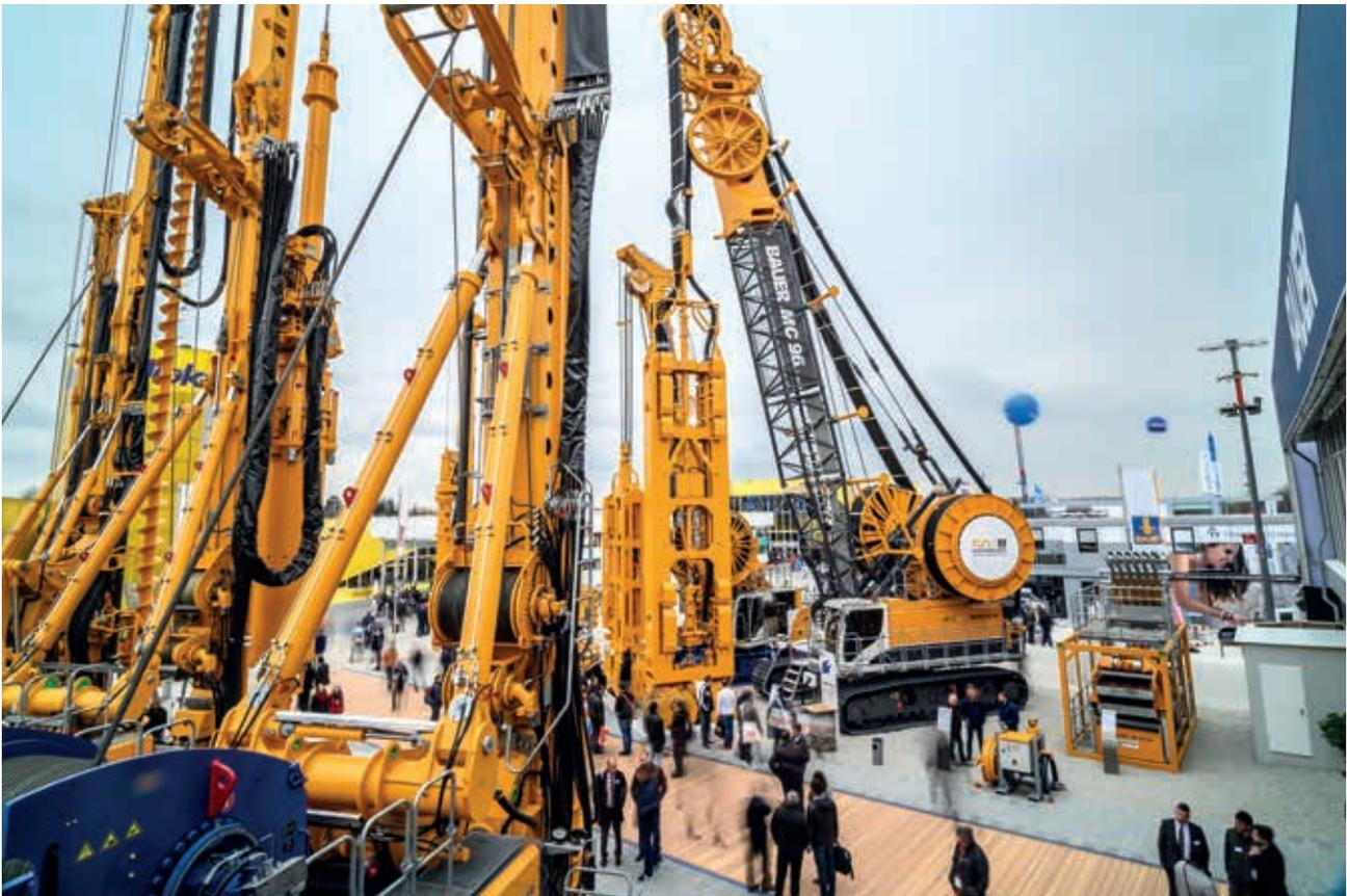
*The 500 kW electric drive of the BAUER MC 96 duty-cycle crane has decisive advantages over an internal combustion engine: It does not produce any local exhaust gases and noise levels are significantly lower.*
