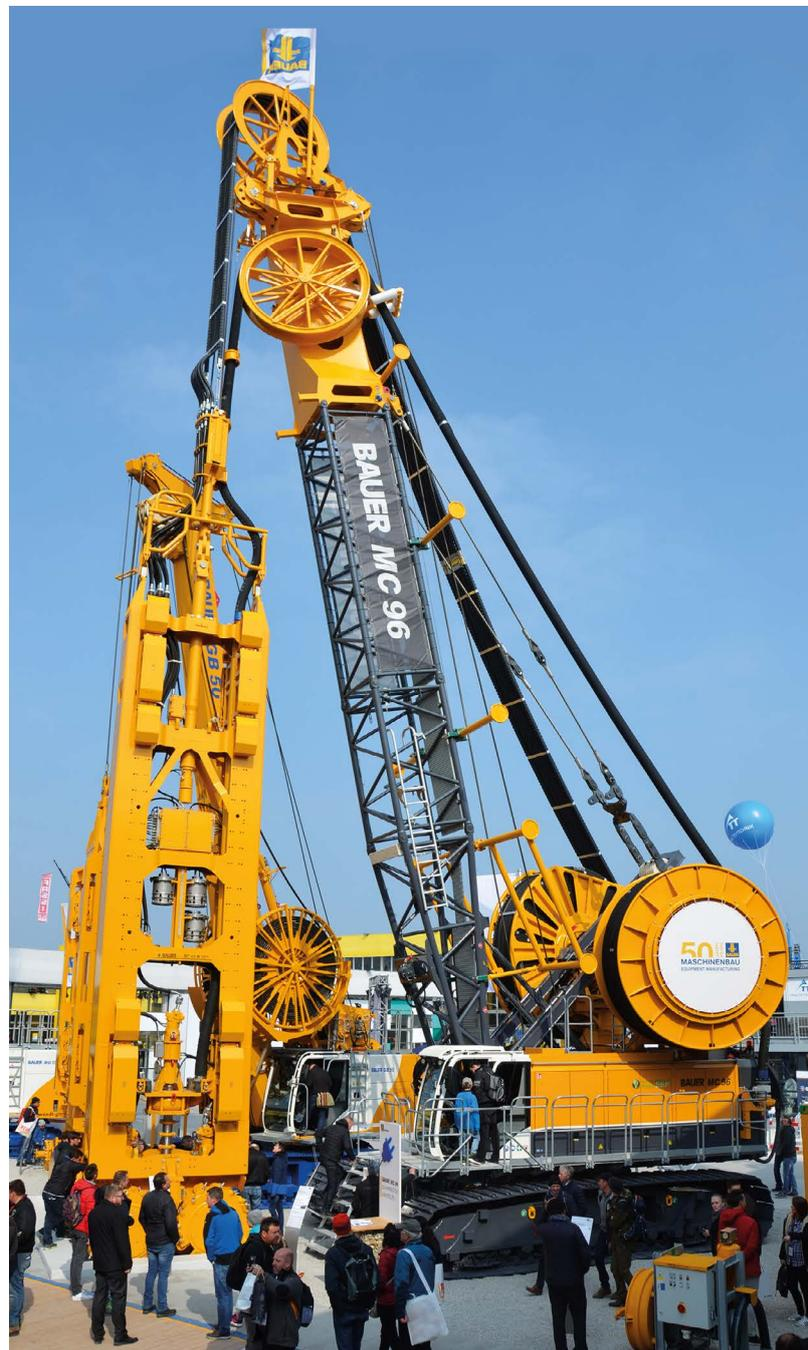
*At Bauma 2019 in Munich, BAUER Maschinen GmbH presented the first electrically driven cutter based on a Bauer duty-cycle crane.*
