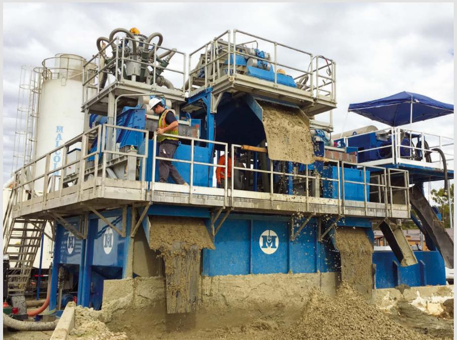
**USA** In Wilmington, Malcom Drilling Company used a BE 550 desanding plant for trench cutters. **top**
