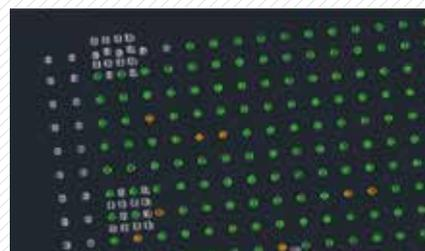
*Graphical verification of quality criteria. In this example, degree of completion and compliance with drilling depth requirements.*
