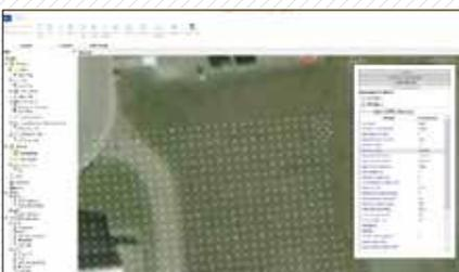
*Georeferenced summary of pile element properties such as planning parameters, production parameters, quality tests and logs.*
