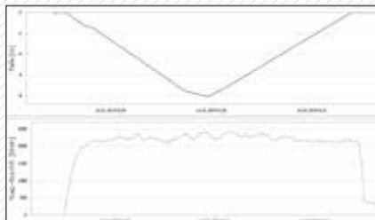
*User interface of the b-project data management software with analyses of drilling depth and suspension flow rate.*
