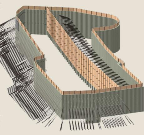
3D model of an excavation pit with pile wall tied back with anchors.
