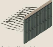
Part of a model: pile wall with I-beam shoring and anchor layers.
