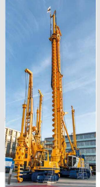
pact transport dimensions. The completely revamped BT 50 base carrier offers an array of advantages: The integrated service platform enables easy access to all service points in the uppercarriage while meeting the highest standards of occupational safety. The BG 15 H also features impressively low noise emissions and outstanding fuel efficiency.
