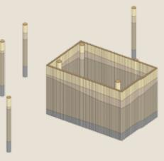
Derivation of soil stratification and excavation quantities in the CAD system.
