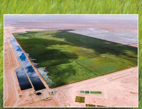
Reed has been growing in the first section of the treatment plant since 2011 (large image). Meanwhile, the plant covers a total area of 10.<u>5 km² (small image).</u>
